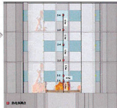
Figure 3(c): Temperature Measurement Points outside the Wooden Boards and Windows
