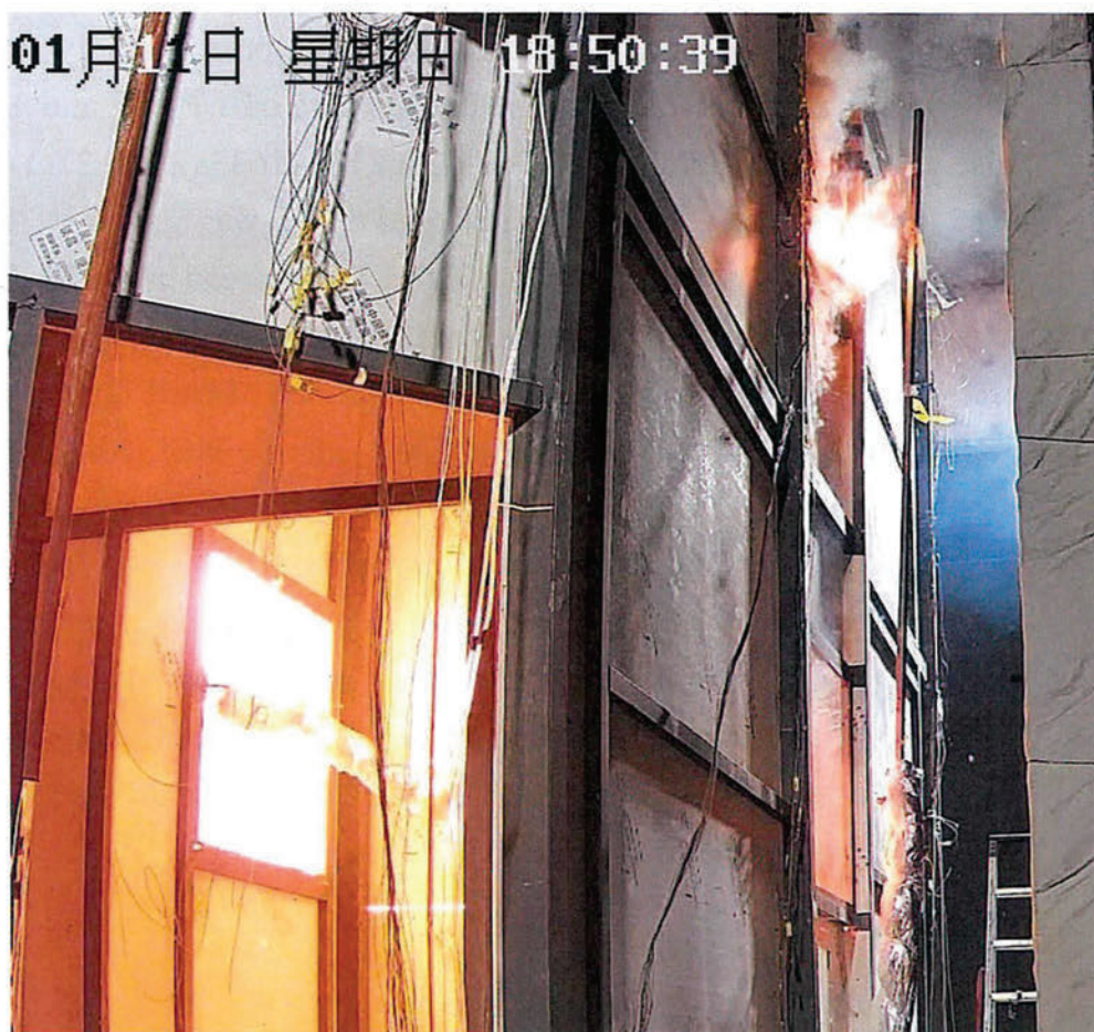
Photo 3(b): The Wooden Board on 2/F Ignited
