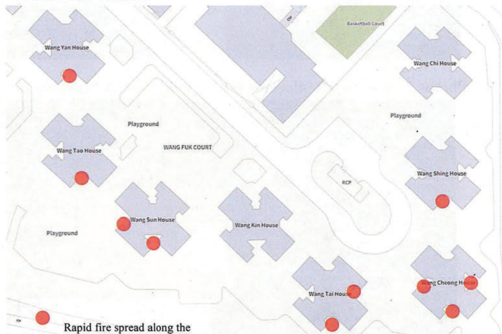
Figure 2: Rapid Fire Spread along the Re-entrants
