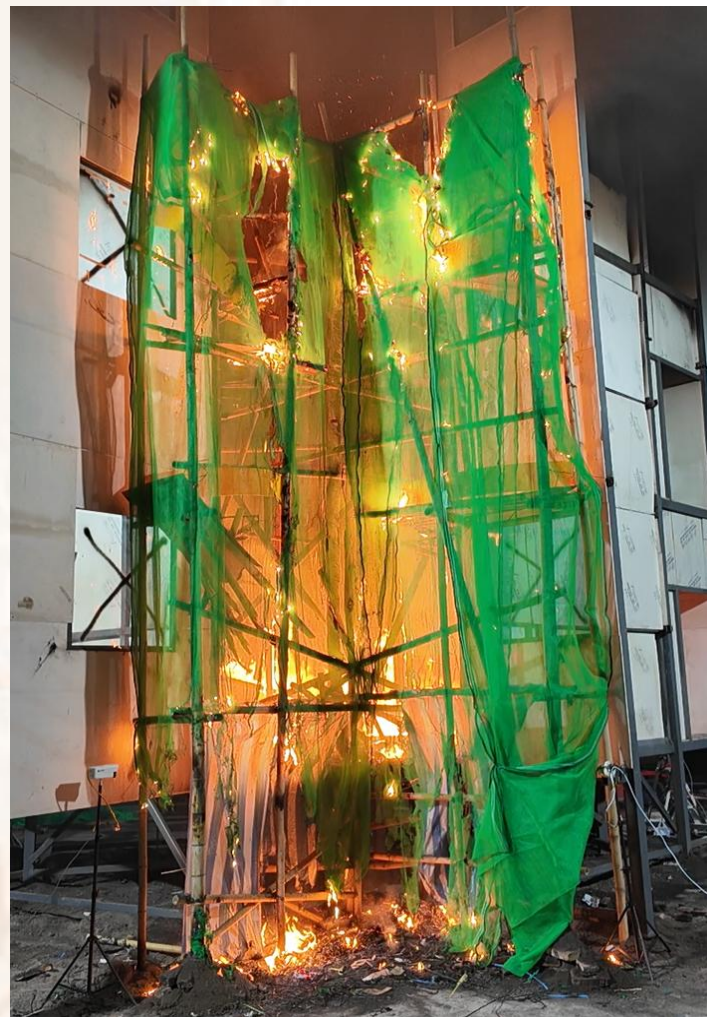
Fire Spread along Safety Nets in Test 13
