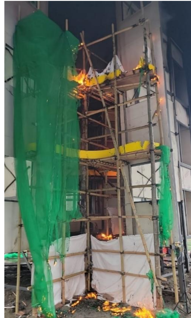
Fire Spread along Safety Nets in Test 12
