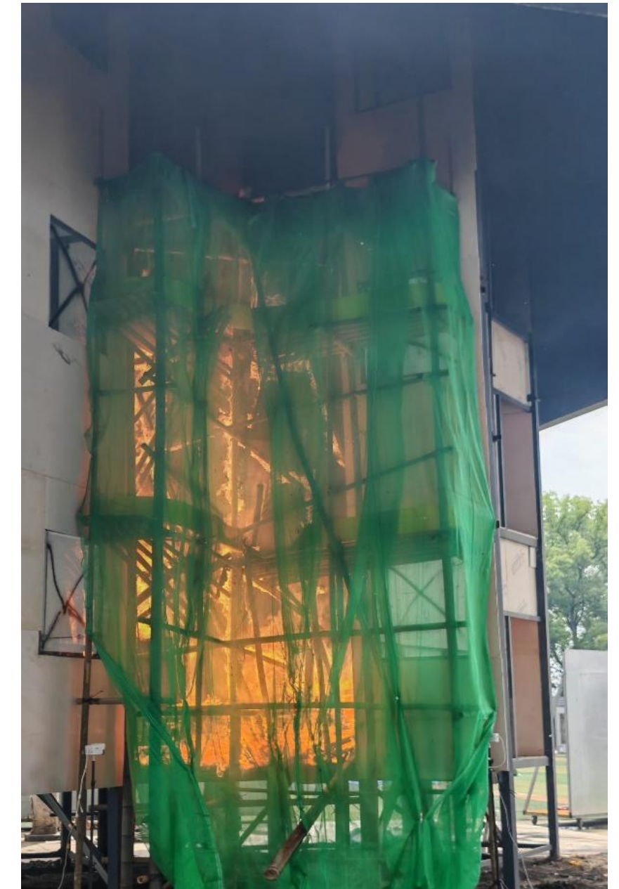
Full Developed Fire in Test 8 using non-FR Safety Nets
