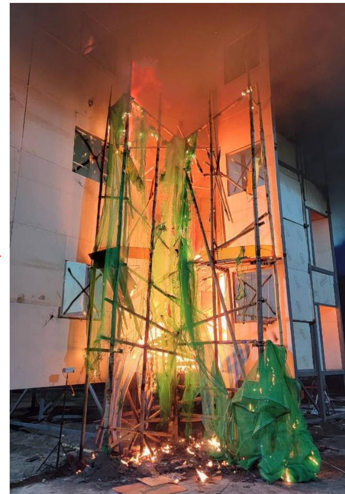
Fire Spread along Safety Nets in Test 13
