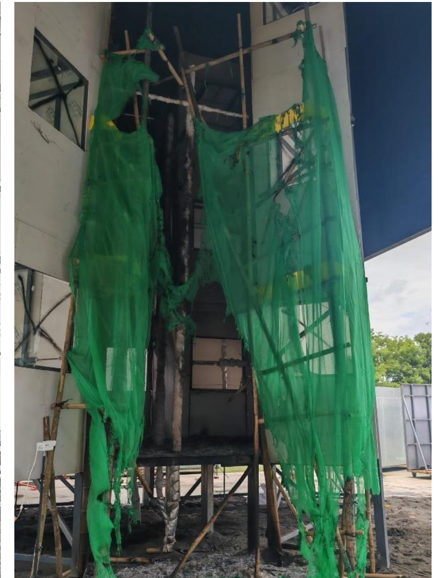
Post Fire Fire in Test 8 using non-FR Safety Nets
