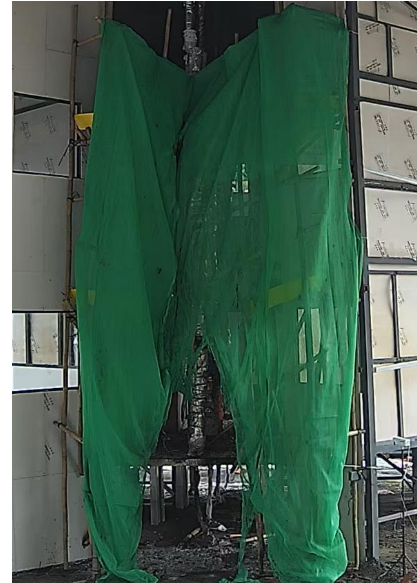
Post Fire Condition in Test 4 using FR Safety Nets
