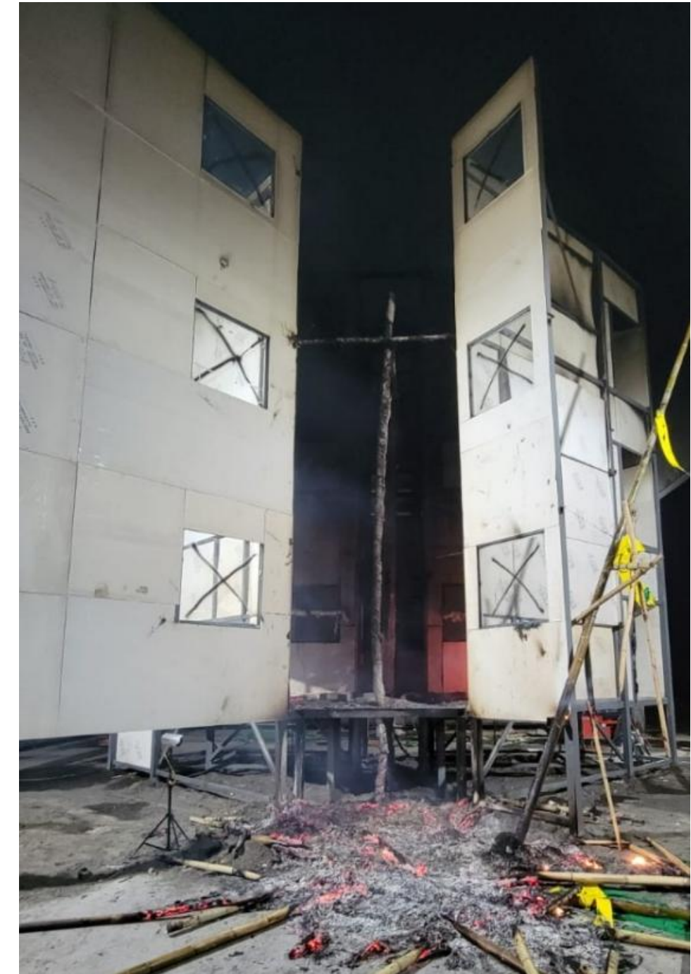
Post-Fire Condition in Test 13 using Safety Nets collected from Wang Chi House and non-FR Canvas
