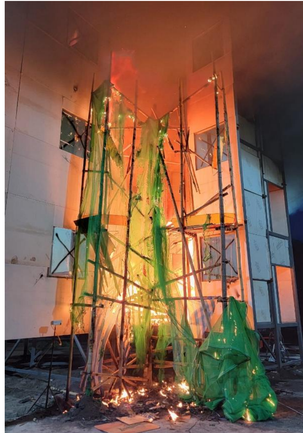
Fire Spread along Safety Nets in Test 13
