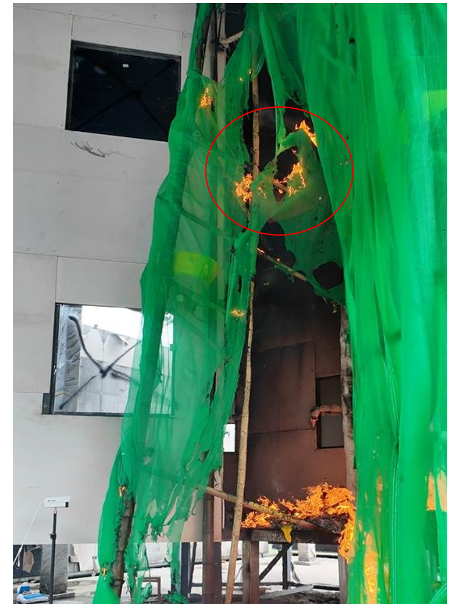
Fire Spread to Other Construction Materials in Test 8
