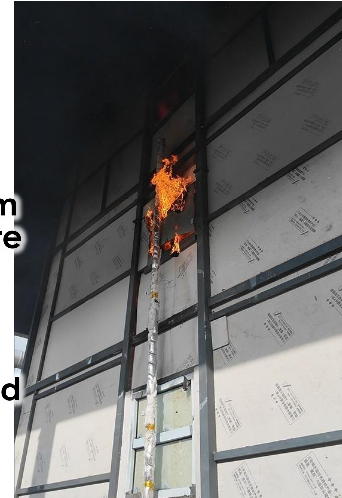
Ignition of Aluminium Composite Panel (7 min 49 sec)
