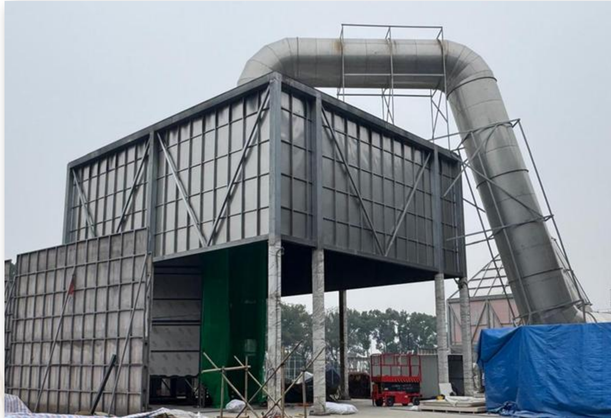
The Mega-Scale Cone Calorimeter at Sichuan University of Science and Engineering (SUSE) 四川輕化工大學
