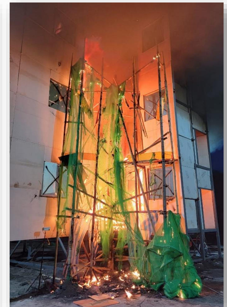
Test 13 using Safety Nets collected from Wang Chi House and non-FR Canvas
