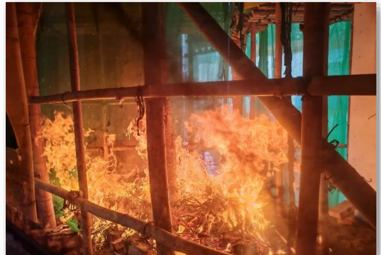
Fire Developed from a Small Fire Source During Fire Tests
