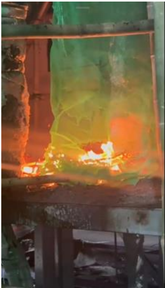
Photo 6-14 (c) & (d): No Spread of Fire along FR Safety Net Observed
