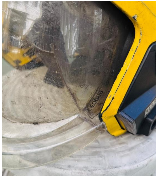
Photo 7-16 (b): Crack on Visor
