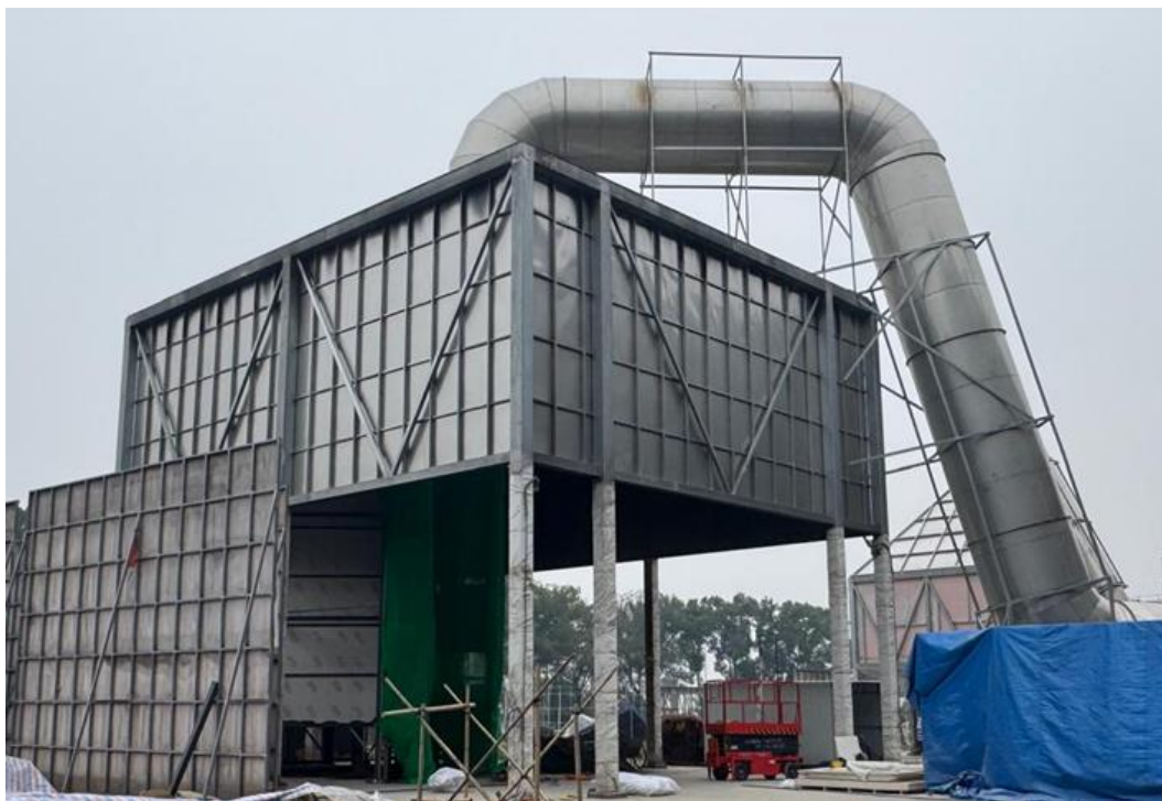
Photo 6-12 (a): The Mega-scale Cone Calorimeter
