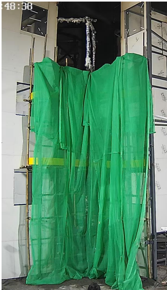
Photo 6-14 (c) & (d): No Spread of Fire along FR Safety Net Observed
