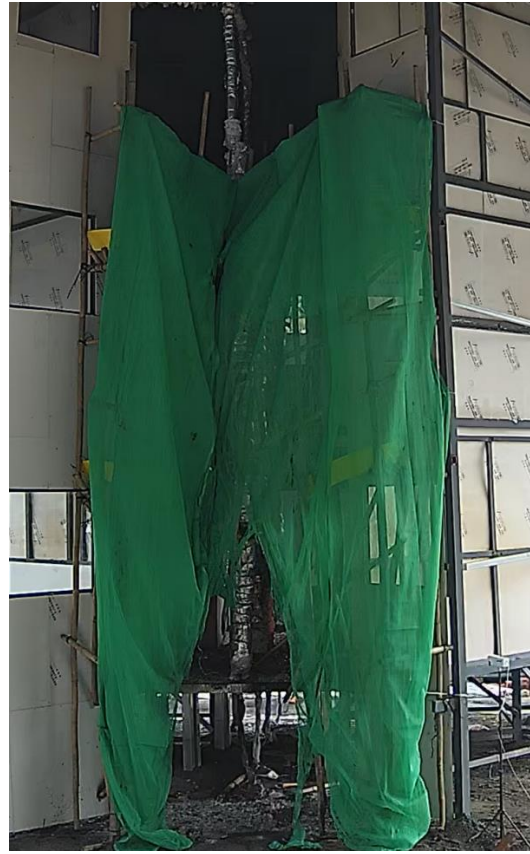
Photo 6-16 (b): No Secondary Ignition Occurred in Test 4
