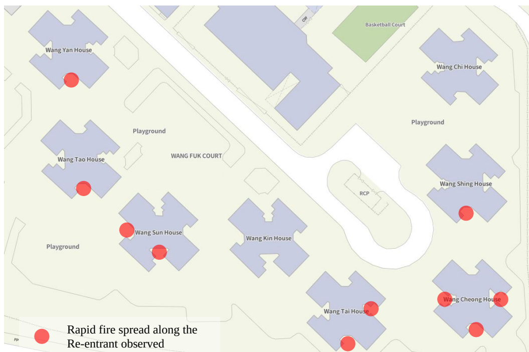
Figure 5-15: Rapid Fire Spread along the Re-entrants
