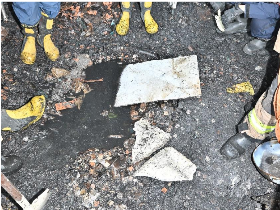
Photo 6-2: Polystyrene Window Covers Found at the Suspected Fire Origin
