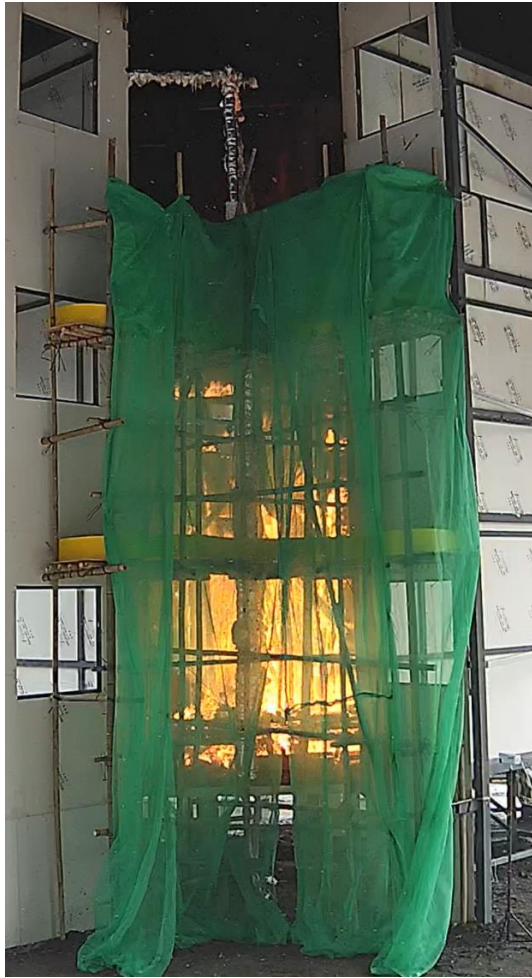
Photo 6-15 (a): Full Developed Fire in Test 3 (Non-FR Safety Net)
