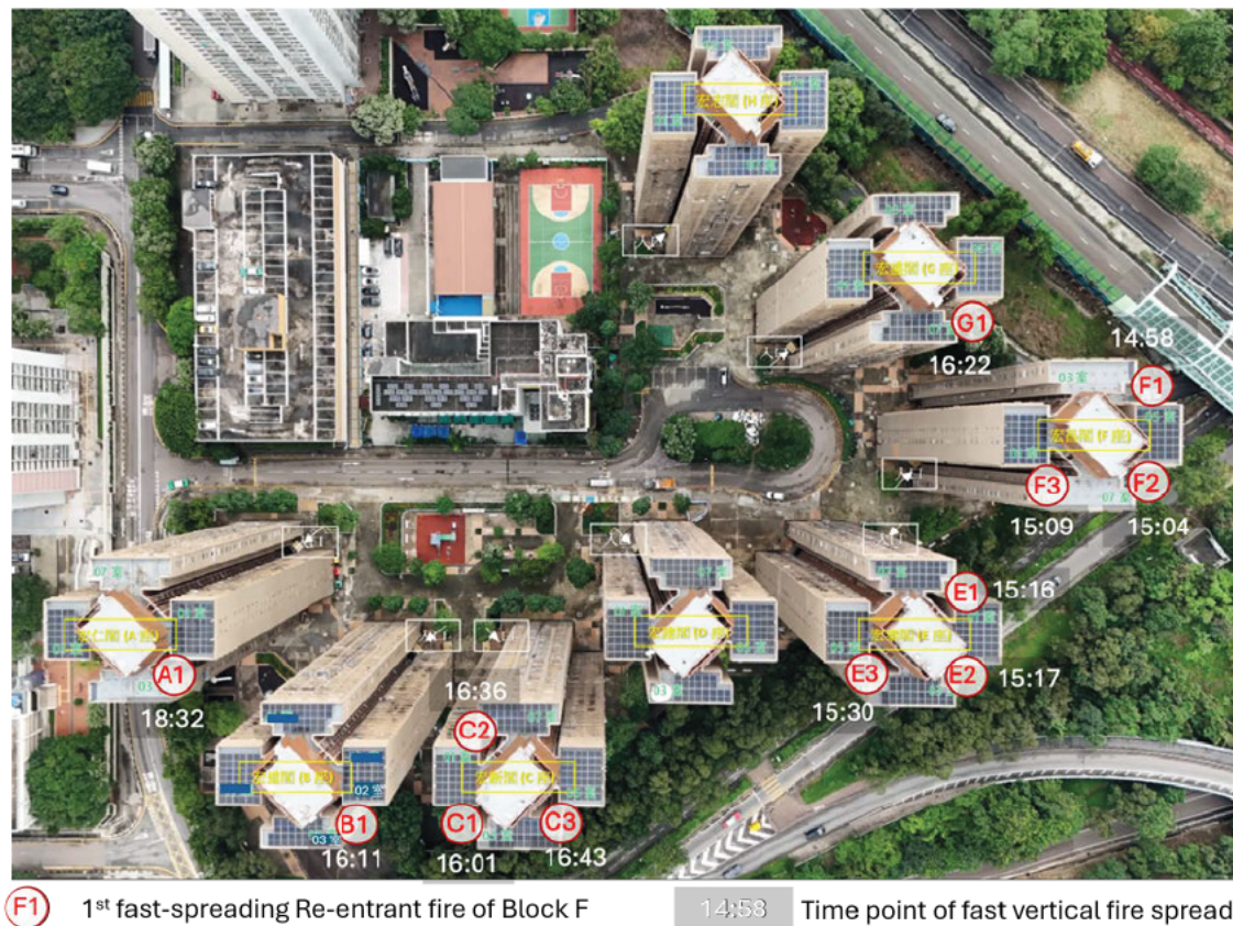
Figure 3-3. Timeline of fast spreading vertical fires at re-entrant regions
