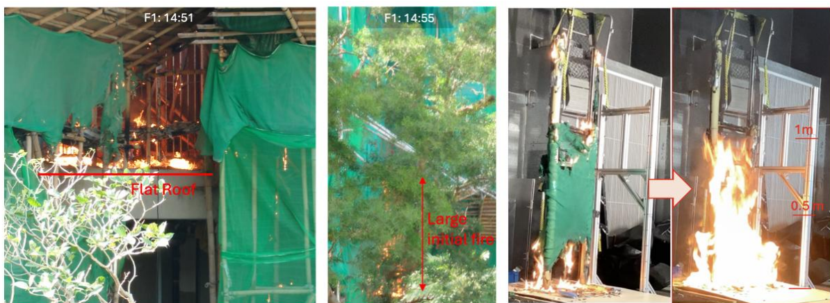
Figure 3-31. Visual evidence of fire initiation VS fire test observations
